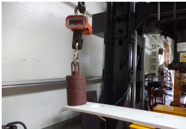
Fig. 10. SSD load in the extreme front position (source: Wielton S.A.)
