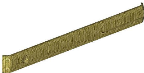
Fig. 2. SSD meshed model - isometric view at the front
