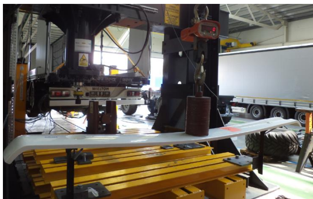
Fig. 11. SSD load in the middle position (source: Wielton S.A.)
