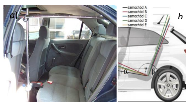
Fig. 3. Viewing the angles of the seat and seat backrest in selected cars
