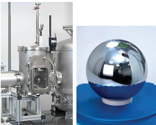
Fig. 2. Vacuum Comparator in PTB and Silicon Sphere [4]
